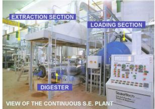
Continuous "Steam explosion" plant of 150 kg/h
