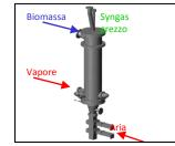
UPDRAFT fixed bed Air/steam 150kWth Coupled with MCI for power generation, Fisher Tropsh
